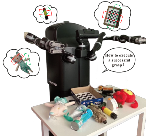
Fig. 1. Kinova MOVO with some novel objects in cluttered scene. Using prior knowledge, it may fail to generate good grasp poses.
